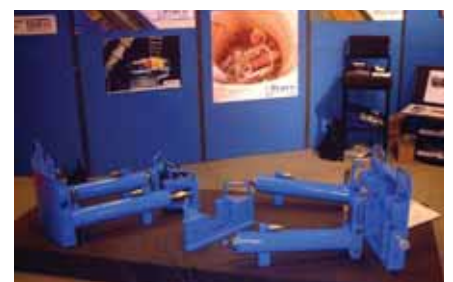
Perco's manhole rodpulling gear
